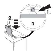
Press the rocker switch (1): green light is on, the machine is now ready for operation.
