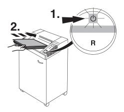
Is the rocker switch pressed? The green light rocker switch is ON? (1.). Insert paper (2.).
