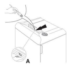
Machine will not stop. Remove plug. Clean the photo cell (A) with a small brush.
