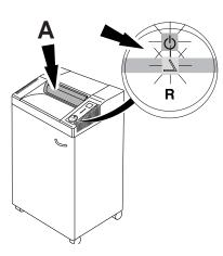
To remove any paper debris from a paper jam, the machine runs for a short Time, reverse with open safety flap.
