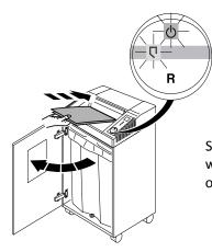
Stops automatically when Front door is opened
