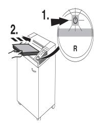
**If required:** Press the rocker switch "R" and remove paper.
