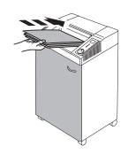
The door must be closed when operating the document shredder!
