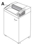
Do not operate the machine without the safety flap (A).
