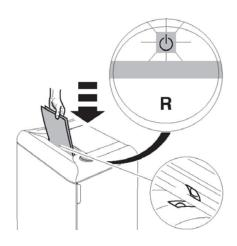
Feed the paper into the centre of the feed opening? (photo cell) (A)
