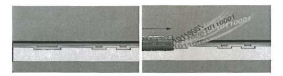
The DX-CD2's technology physically removes the information layer from the CD-ROM permanently and safely while keeping the CD intact.
