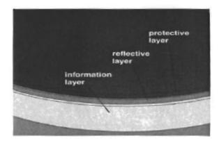
A CD\_ROM is made up of multiple layers: Data resides in the "information layer" of pits and lands. Data is a sequence of 9 unique spaces of lands and 9 unique sizes of pits. Data is imbedded in the polycarbonate.
